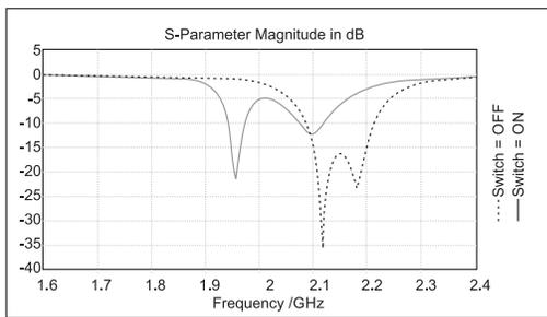
Figure 3: Return loss for ON and OFF states of switch.
