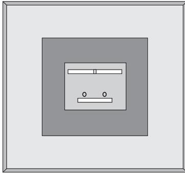
Figure 2: CST model of proposed antenna (when switch is ON).
